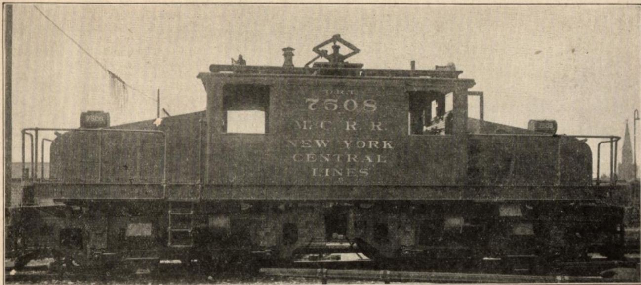
One of the electric locomotives used by the Michigan Central in the twin-tube tunnel which connects Detroit with Windsor, Ont., by speedy rail service under the Detroit River. These efficient locomotives are one of the important factors in the satisfactory all-season transportation provided by the Michigan Central at this point.
