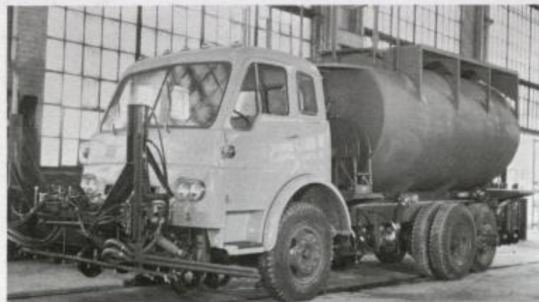
WEED SPRAYER, designed and built at Jackson shop, operates on track, can run on roadway adjacent to tracks, and on the highway.
