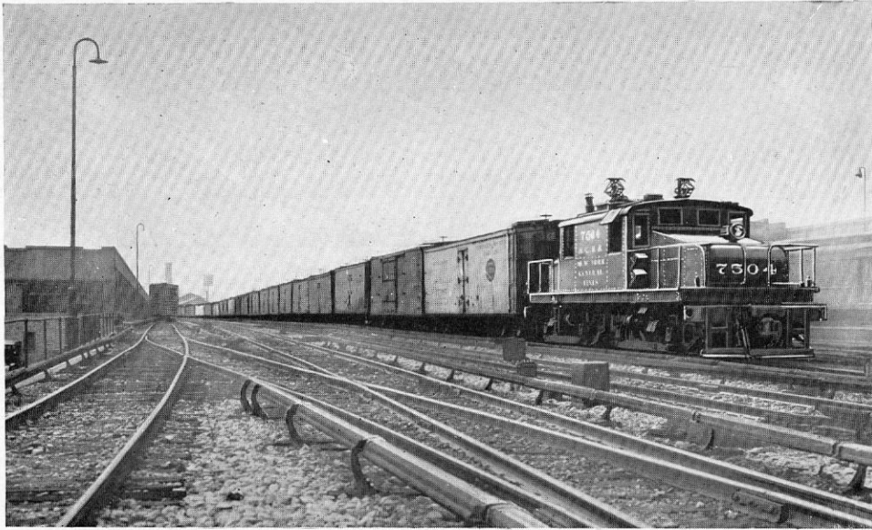
ONE OF THE ORIGINAL 100-TON LOCOMOTIVES PLACED IN SERVICE IN 1910 HANDLING FREIGHT TRAIN IN DETROIT YARDS
