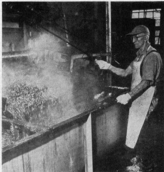
HEAT TREATMENT before pressure is applied kills yeast action and brings out the attractive purple color and familiar odor of the grape juice.
