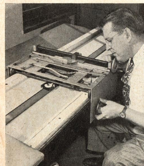
CENTRAL OFFICE in Buffalo, to which all completed tapes are sent, uses instruments to check each against standard for run.*
