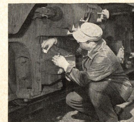
TO GUARD against overheated journals, passenger cars and locomotives are equipped with smoke and odor alarms.*
