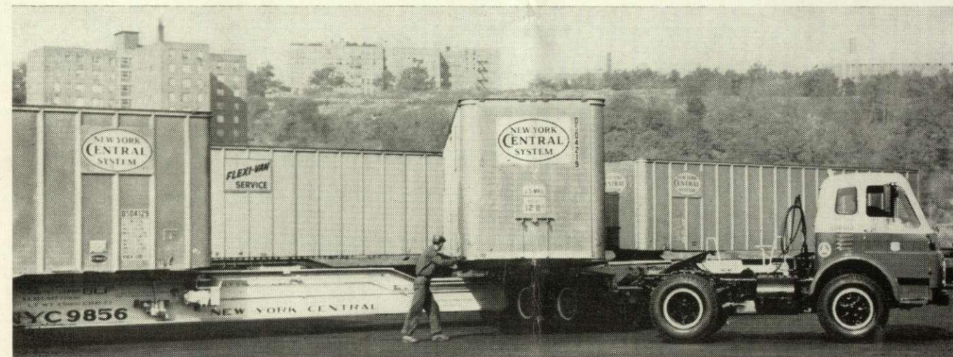
IN LESS THAN FOUR MINUTES A FLEXI-VAN LOADED WITH U.S. MAIL IS TRANSFERRED FROM NYC TO HIGHWAY VEHICLE.
