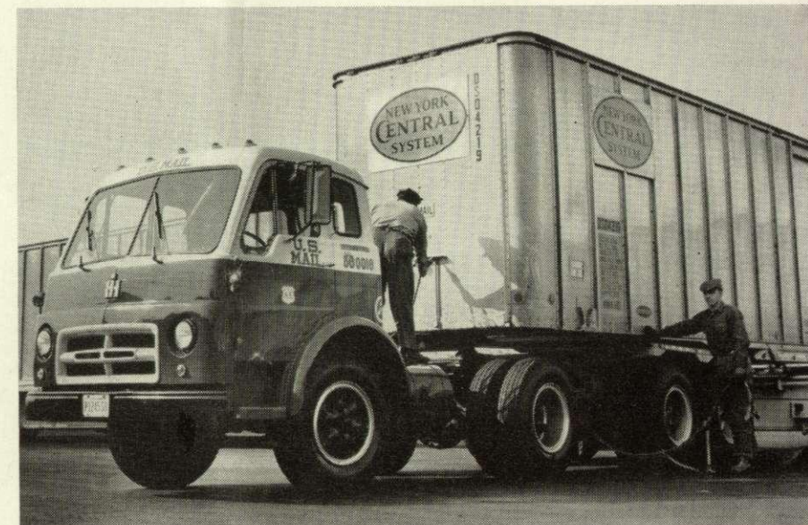
FORTY FOOT FLEXI-VAN is swung into position for coupling with U.S. Mail tractor and movement to intercity postal facility in New York City. Photo above shows Flexi-Van operations in NYC's High Bridge Yard in the Bronx.
